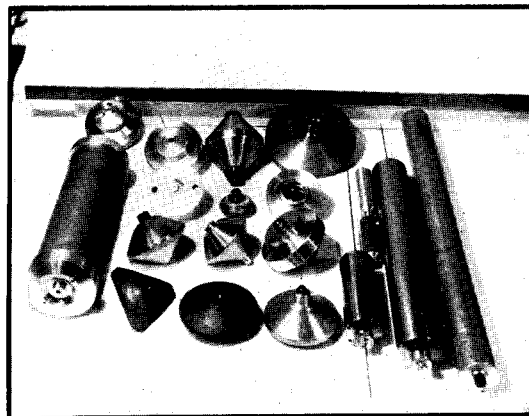
FIG. 13. Photograph of a collection of rotors that have been spun in a vacuum.
